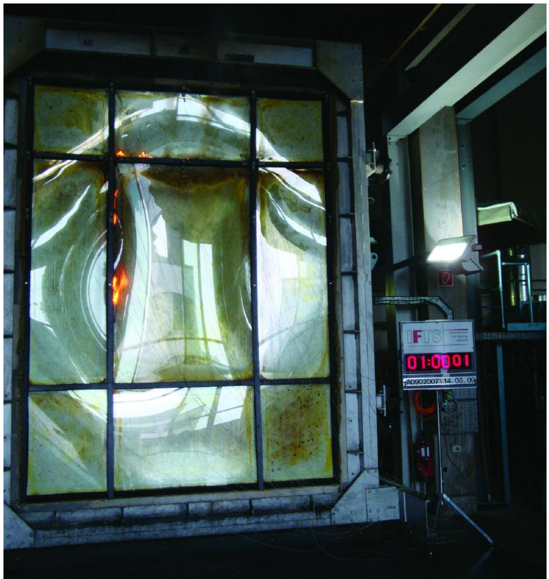
Kawneer's AA®100 FR Curtain Wall Screens are 30 minute Fire Rated. The image above shows the screen damage after 60 minutes exposure.
